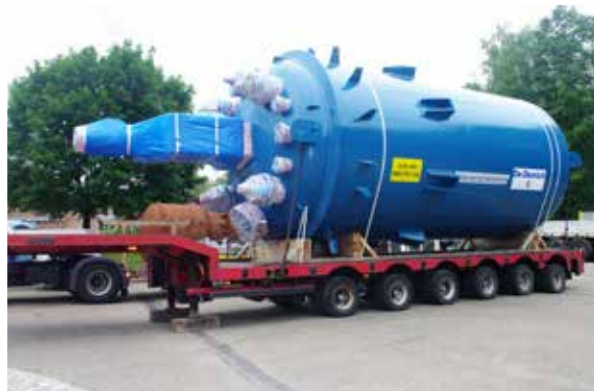
Reactor BE 80m 3
