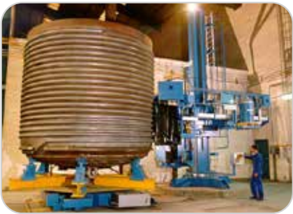
Automatized welding tool
