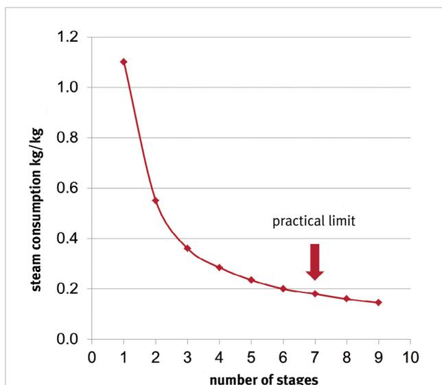
Fig. 2: Steam consumption in a multiple-stage evaporation plant
