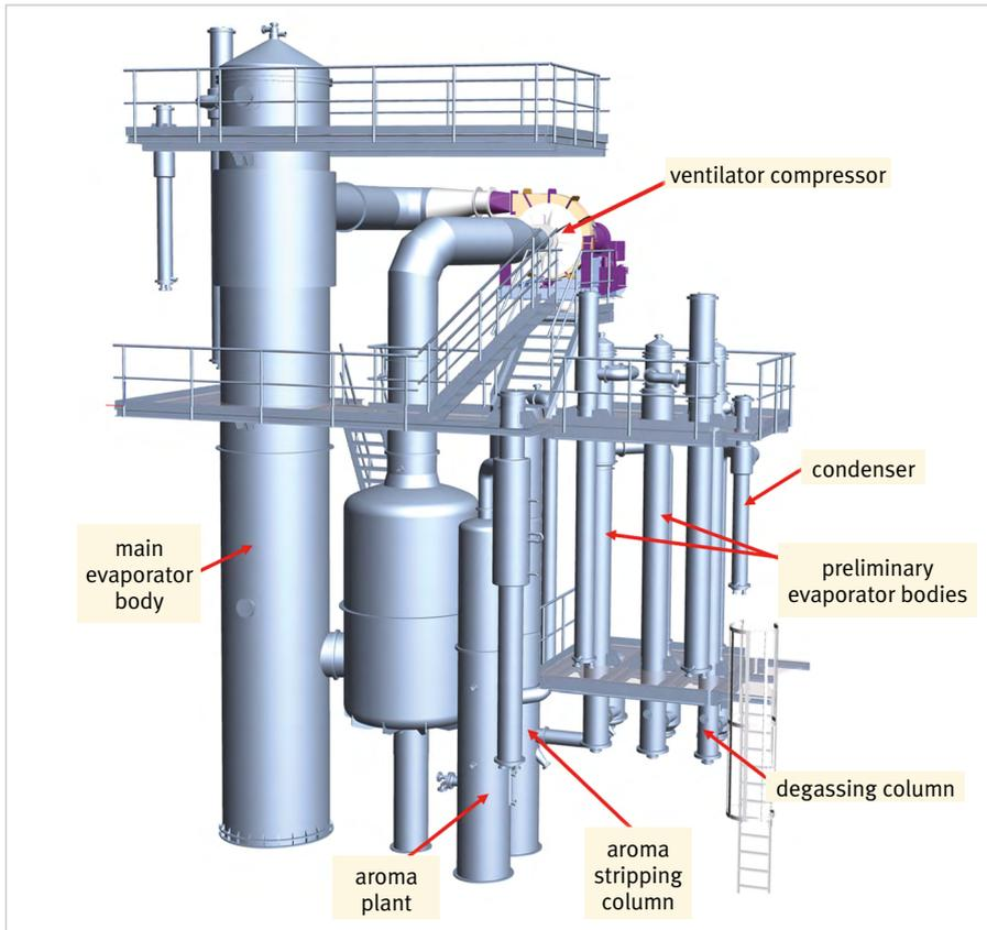
Fig. 6: Aroma recovery / preliminary concentration plant with a 1-stage ventilator compressor.
