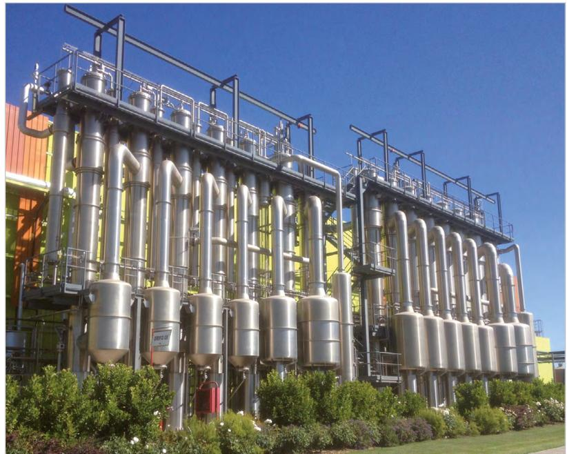
Fig. 1: 6-stage and 7-stage evaporation plants for manufacture of apple-juice concentrate with a water evaporation rate of 25 or 50 t/h.
