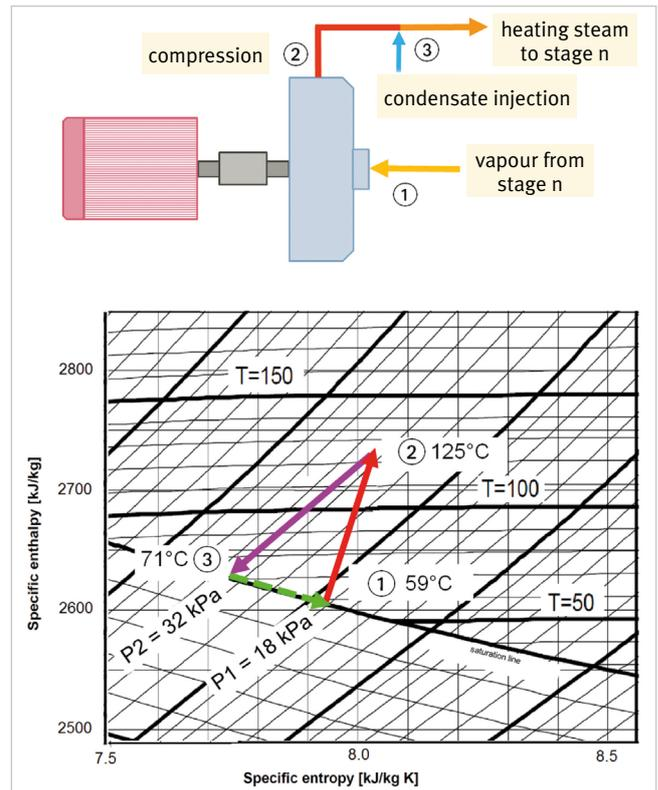
Fig. 4: Principle of mechanical vapour recompression (MVR)
